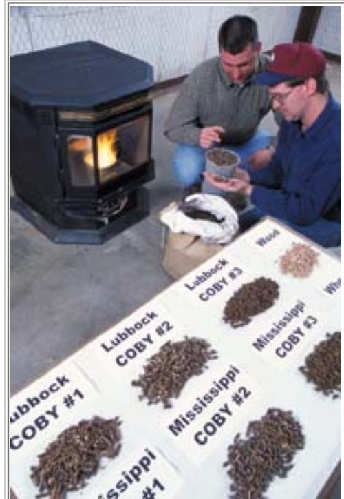
Sanders (left) and Holt evaluate eight different pellet fuels for efficiency, pollutant emissions, and ease of handling.
