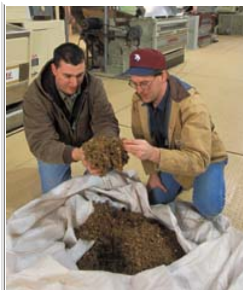
In a cotton gin, Sanders (left) and Holt examine extruded cotton gin waste before it is made into pellets for use as feed, fuel, or fertiliser.
