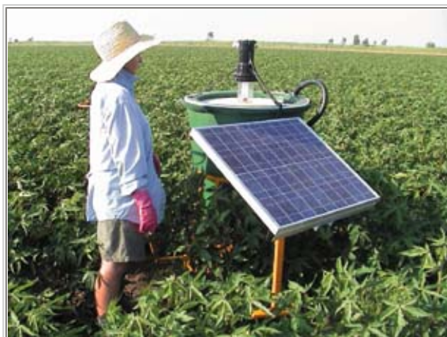
Leah MacKinnon checks one of the solar powered array of light traps.
