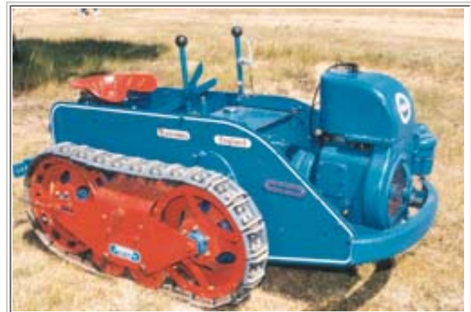
A Ransomes MG 5 crawler magnificently restored by Maureen Creasey of WA. The MG 5 was not fitted with hydraulics and three point linkage so the rear implements had to be raised by the large hand lever located on the right side of the operator. Note the throttle control and stop button on the left hand steering lever. (Photo IMJ.)
