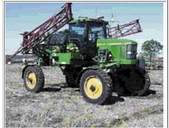
GPS and radio antennae on spray rig.
