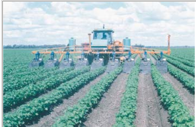
A recently-released, weed-activated sprayer which uses video imaging to target weeds. This model is designed for shielded, inter-row spraying.
