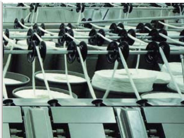
Cotton slivers entering the Murata Vortex Spinner.
